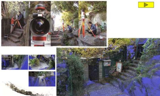
Input Terrestrial LiDAR data : RIEGL VZ-400
